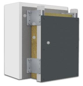
Structural Back-up Wall (by others): Steel or wood frame with glass mat gypsum sheathing in compliance with ASTM C1177 or code compliant OSB or plywood sheathing, concrete or core filled concrete masonry, existing structurally sound, uncoated brick or other masonry wall construction.
